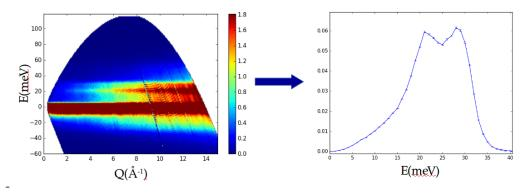
The multiphonon package takes the inelastic neutron scattering spectrum, shown on the left, and produces the phonon density of states shown on the right.
