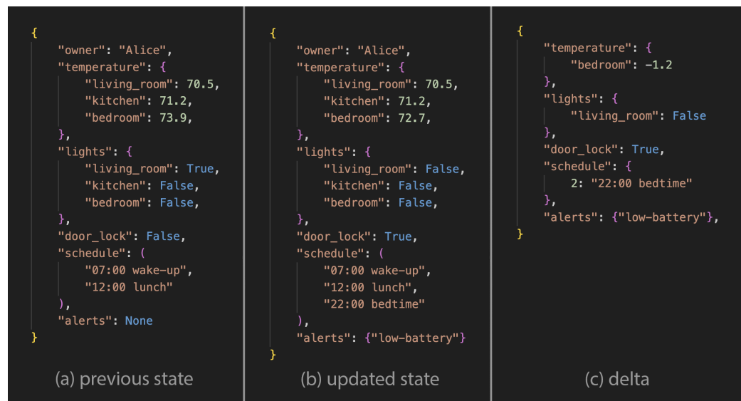
Figure 3: An example of human-readable change tracking with KeepDelta. (a) Previous smart-home state. (b) State after updates to temperature, lights, door lock, schedule, and alerts. (c) Delta produced by KeepDelta, which records only the changes including numeric adjustments, boolean toggles, a tuple insertion, and a new set element, offering a concise, easily interpretable summary.
