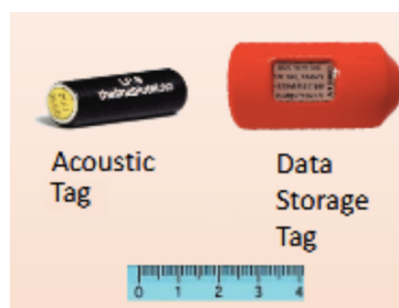
Figure 2: Example of an acoustic tag (on the left) and a DST (on the right). See the centimeter scale for size reference.
