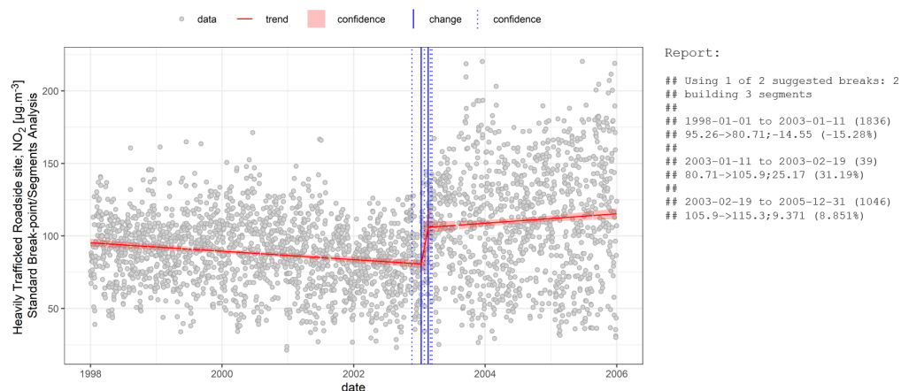
Figure 2: Standard AQEval break-point/segment analysis (graphical output and report) of an \text{NO}_2 1998-2005 time-series from a heavily trafficked roadside in the UK.
